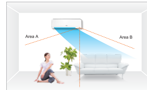
If a person is detected in area A, airflow is directed toward area B.
