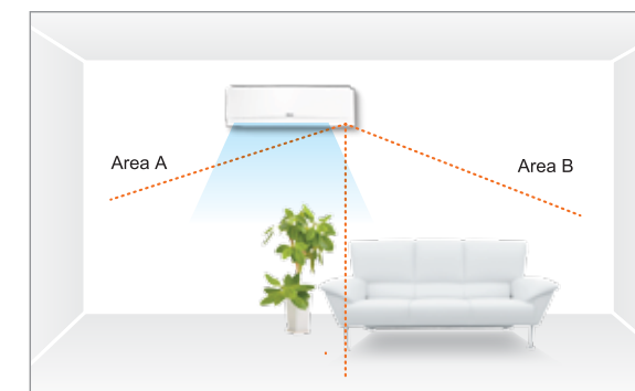
If no one is detected in either area A or B for 20 minutes, Intelligent Eye automatically adjusts the set temperature.
